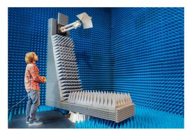
At the heart of the facility is a world-class state-of-the-art spherical near-field RF test chamber that significantly enhances our measurement capabilities, and in many cases enables the company to exceed clients' needs and expectations.
